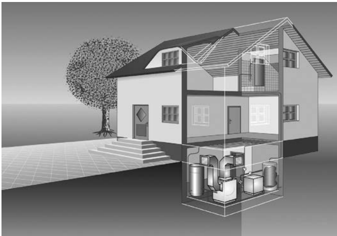
Figure 5.35 Air-water heat pump
